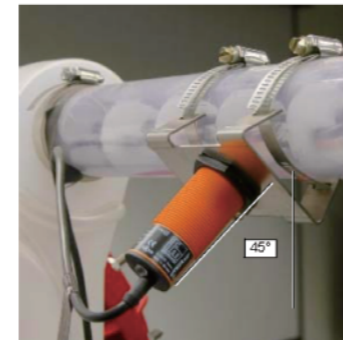
传感器 Material Line Sensor
