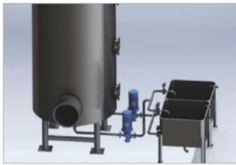
循环喷淋系统 The Circulating Spray System
